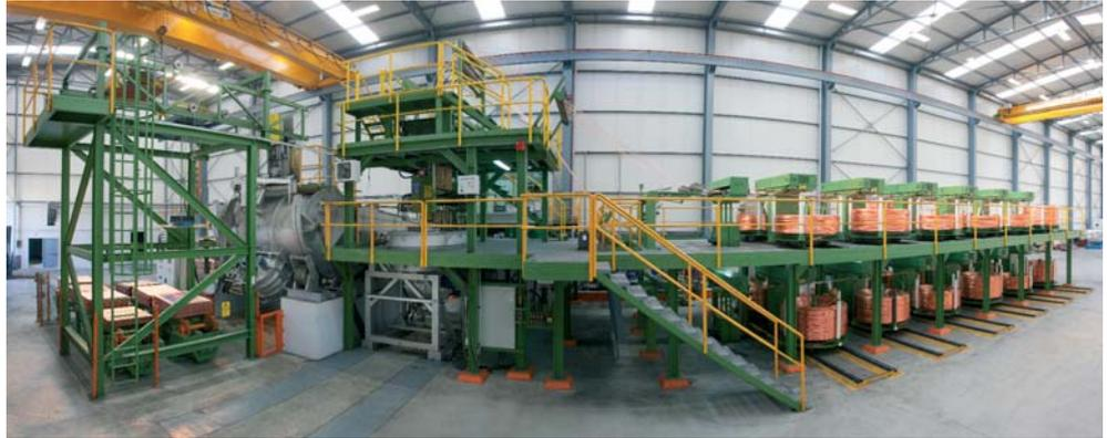
**UPCAST® technology is available in both single- and double-furnace configurations. Single-furnace lines are compact units built around a combined melting/holding furnace while double-furnace UPCAST® lines comprise of separate melting and holding furnaces connected with a launder. Shown here is a double-furnace UPCAST® unit with a production capacity of 24,000 TPA.**
