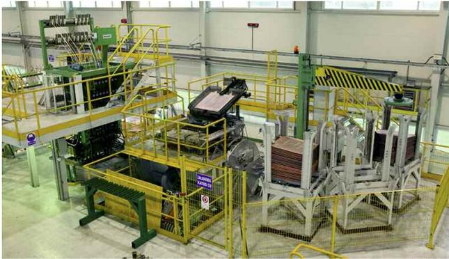
This feature set is in large part the result of UPCAST OY's painstaking attention to careful design, which unites the process steps through an advanced, highly automated control system that allows operators to cast different copper rod sizes simultaneously while adjusting production
