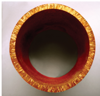
Cross sections of cast tubes: a) Conventional UPCAST®; b) UPCAST®-SGTube
