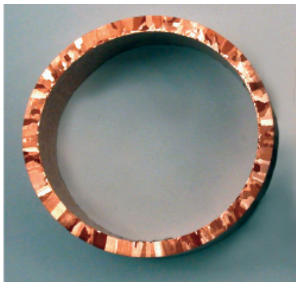
Cross sections of cast tubes: a) Conventional UPCAST®; b) UPCAST®-SGTube
