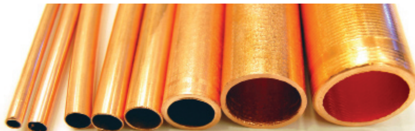
Cast tube (far right) and several drawing steps
