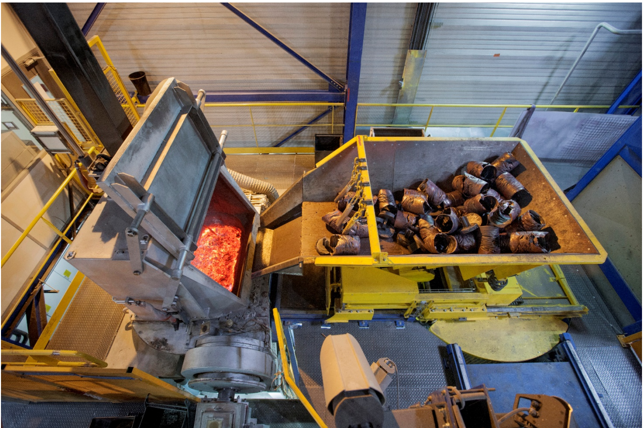
Gindre Duchavany, France - First UPGAST® line utilizing 100% recycled copper as raw material. Scrap charging - Photo courtesy of UPGAST OY
