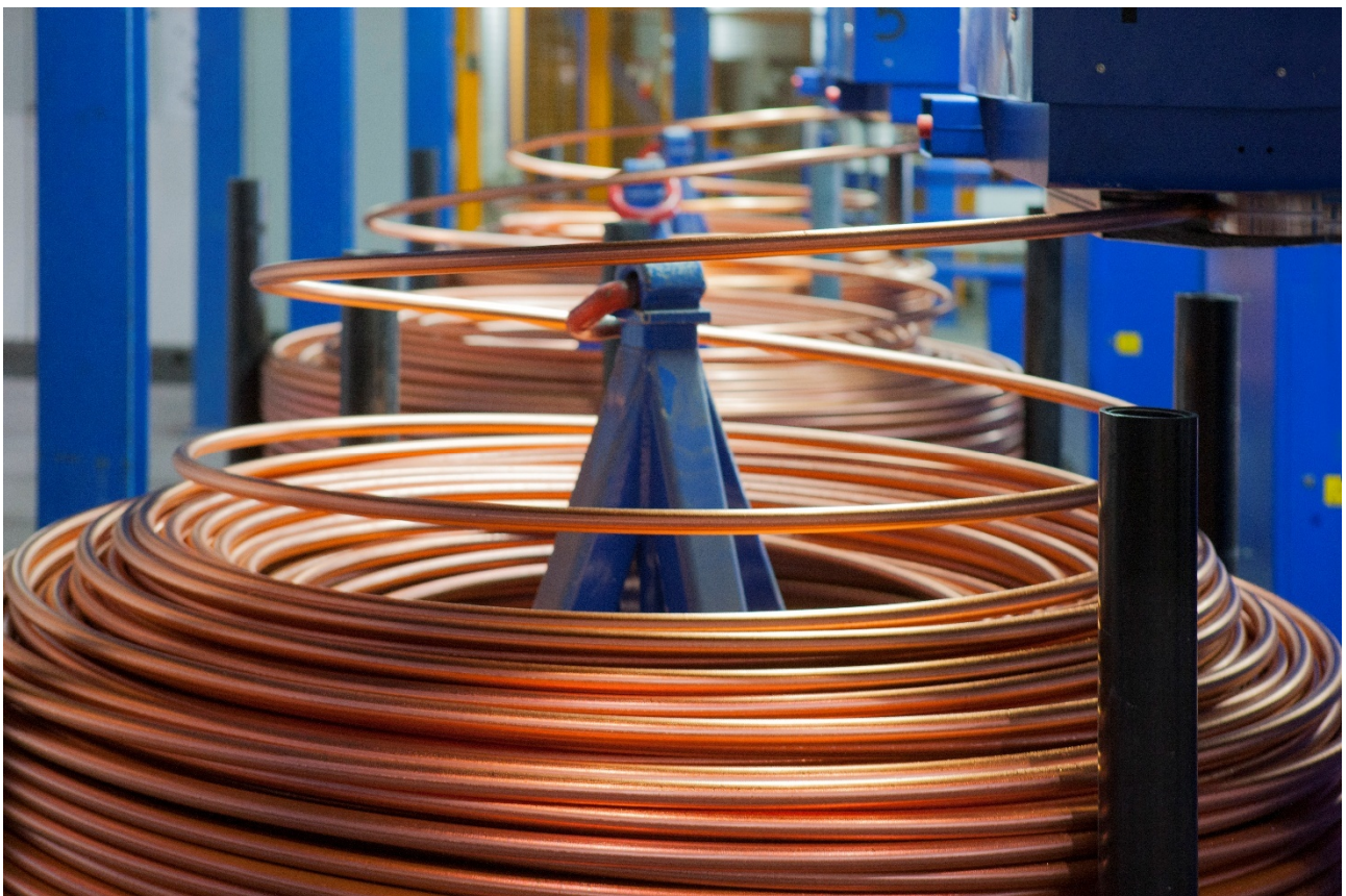
UPCASt® double coilers coiling 25mm rod made from 100% recycled copper - Photo courtesy of UPCASt OY
